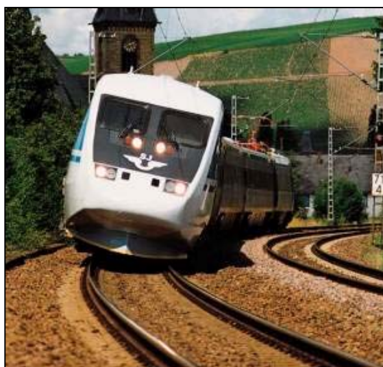
Figure 5: Swedish X2000 tilting train, top speed 200 km/h (Keating, 2000)
