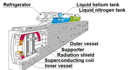
Figure 3. Yamanashi Superconducting Magnet [13]
