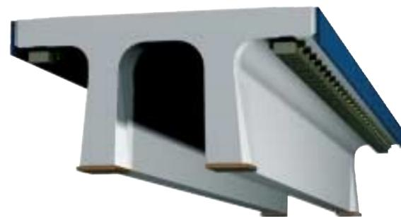
Ground-level guideway developed by Max Bögl
