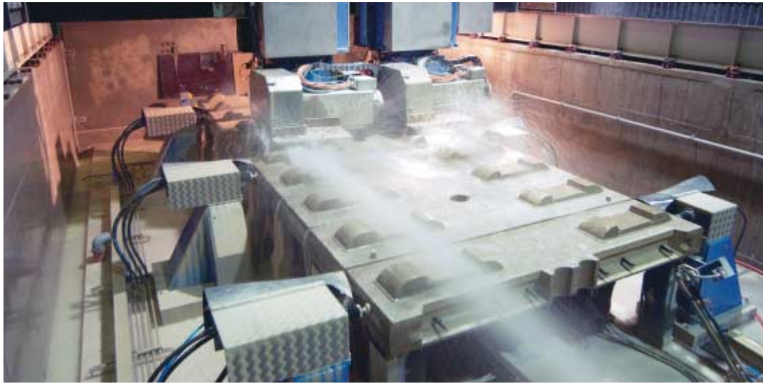
Grinding of the rail geometry into the rail support points of the slab track system Bögl
