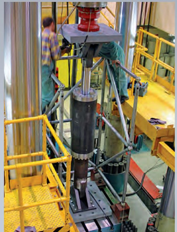
Testing a MAURER hydraulic damper at an independent test laboratory
