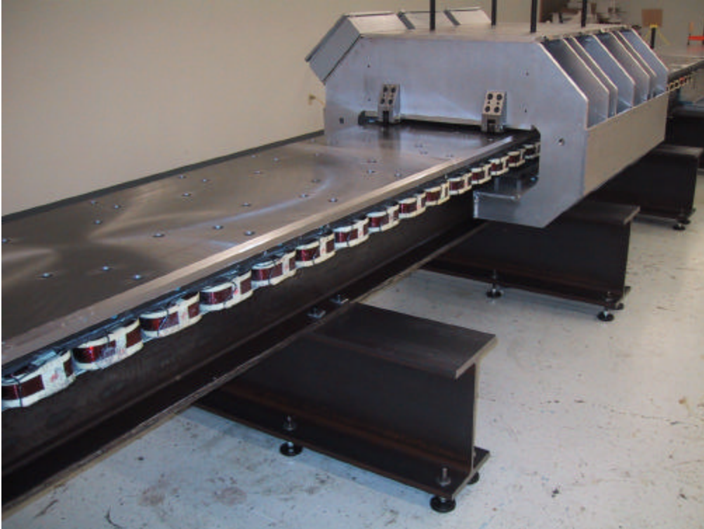
Fig. 9.1. Photograph of prototype vehicle and guideway.
