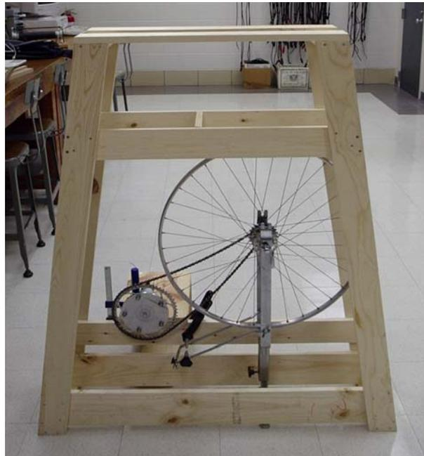
*Figure 9.3 Wheel Attached to Motor*
