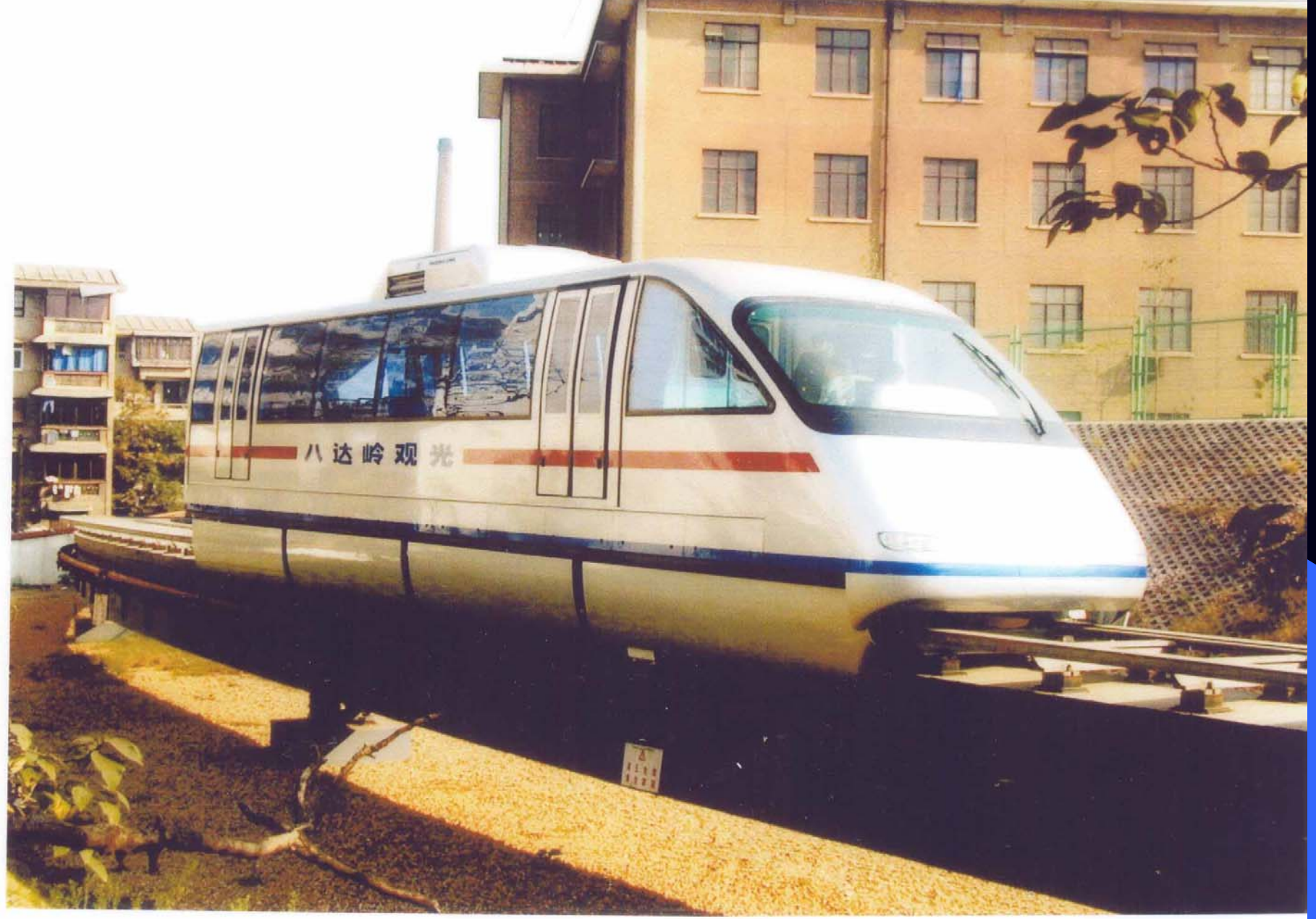
The low speed Maglev CMS-03 test vehicle
