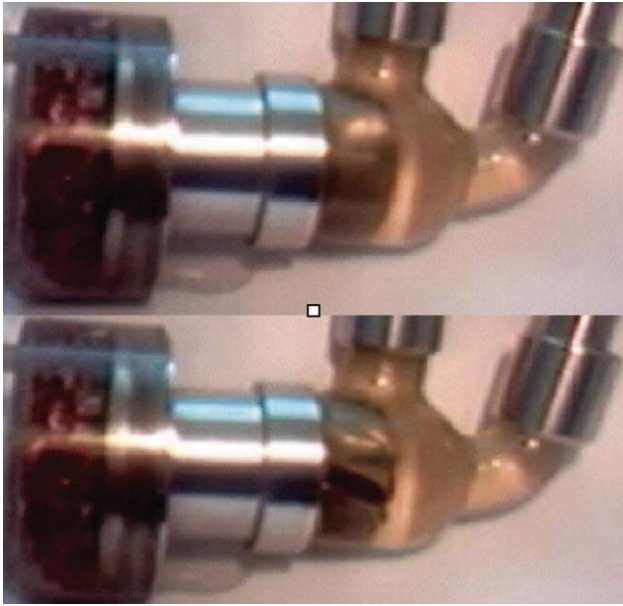
Fig. 4. The driven magnets disc is levitating axially (upper) during rotating at high speed and contacting the spacer (lower) during standstill. The space (black ring) between motor coil and rotor magnets disc at left side of the disc is 0.5 mm bigger in upper than that in lower.
