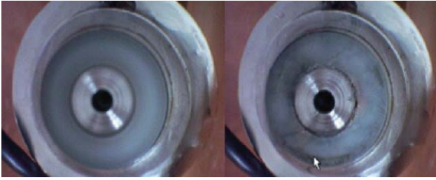
Fig. 7. The rotor keeps concentric with stator during rotating (left) and eccentric at standstill (right), indicating the rotor is levitated during rotation and affiliated to the stator at standstill.
