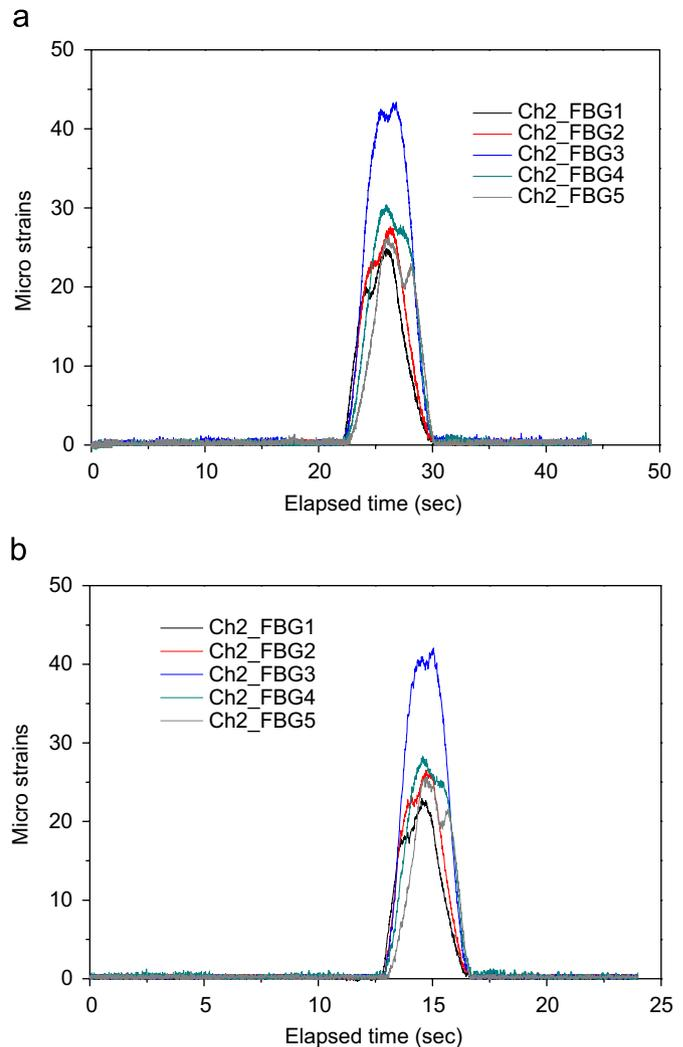
Fig. 6. Time history of bottom strains measured from guideway girder: (a) maglev speed = 20 km/h and (b) maglev speed = 40 km/h.
