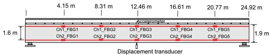
Fig. 4. The layout of sensor locations: (a) cross-section and (b) front view.
