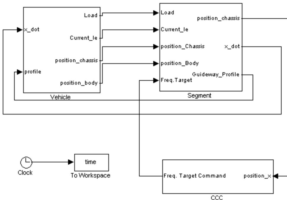
Fig. 3 The MagLev system (the highest level)
