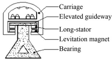
**Fig.1 Suspensive and propulsive magnets in Shanghai EMS-MAGLEV commercial line**
