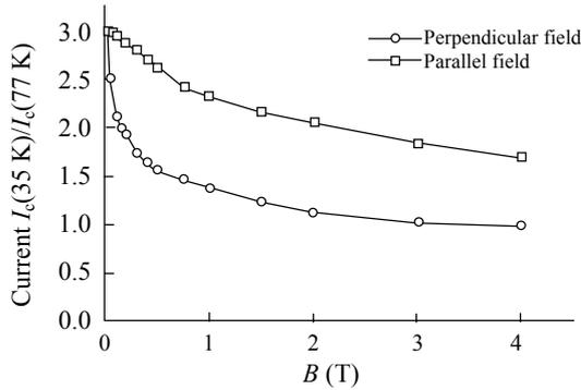
Fig.6 The  $I_c$ - $B_c$  curves of Bi-2223 HTS tape
