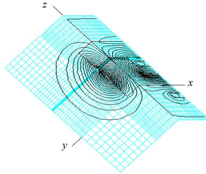
**Fig.9** The flux linkage distributed on the symmetric surfaces of the HTS coil magnet
