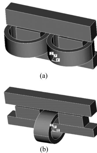
**Fig.3 Structure of Maglev system magnet**
