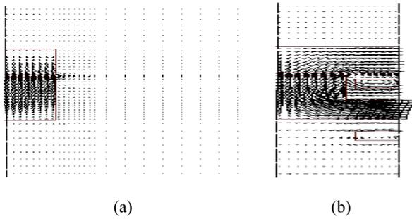
**Fig.8** The flux density distributed on the symmetric surfaces of the HTS coil magnet
