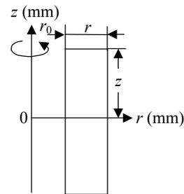
Fig.5 The cross sectional dimensions of HTS coil
