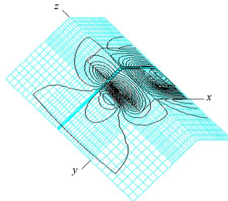
Fig.7 The flux linkage distributed on the symmetric surfaces of the copper coil magnet
