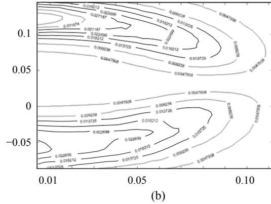
**Fig.10** The contour of flux density components distributed in the partial region of  $yoz$  surface in Fig.3b. (a)  $B_y$  contour; (b)  $B_z$  contour
