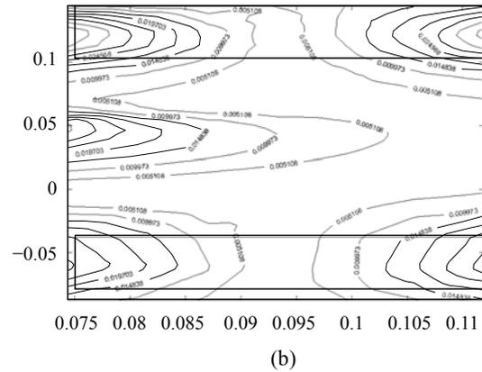
**Fig.11** The contour of flux density components distributed in the partial region of  $xoz$  surface in Fig.3b. (a)  $B_y$  contour; (b)  $B_z$  contour
