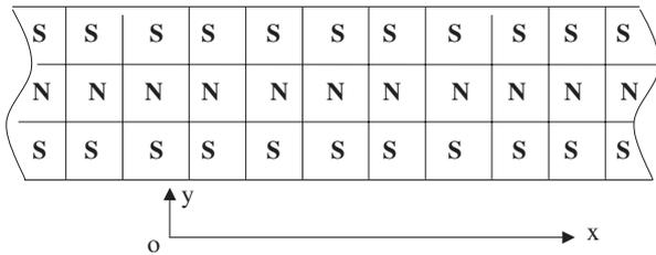
**Figure 2.** Schematic diagram of the track of the Maglev model using small magnets of size  $10 \times 10 \times 10 \text{ cm}^3$ . The magnetic field distribution is uniform along the  $x$  axis and with a larger field gradient in the  $y$  direction.
