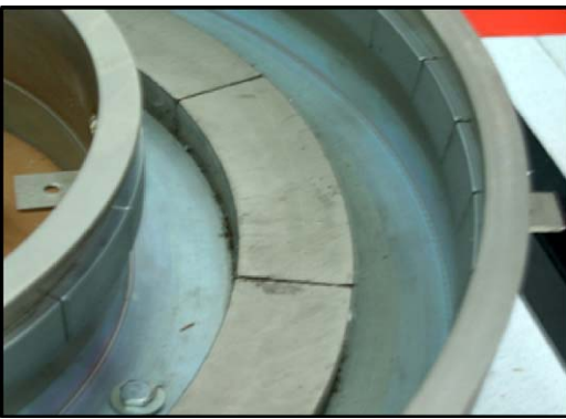
Fig. 4. Detail of side rims of magnetic track.
