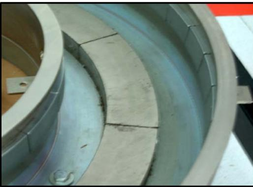
Fig. 4. Detail of side rims of magnetic track.
