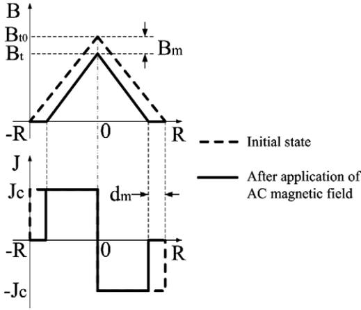
Fig. 1. Distributions of the trapped magnetic field  $B$  and current density  $J$  in the bulk exposed to AC magnetic field.
