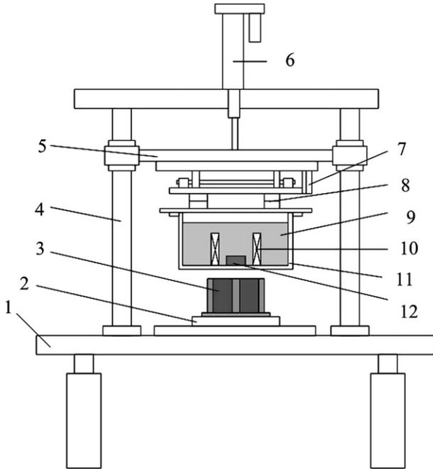
Fig. 2. Schematic drawing of the experiment system. (1) base, (2) lateral drive platform, (3) NdFeB guideway, (4) vertical guide way, (5) vertical drive platform, (6) servo motor, (7) guidance force sensor, (8) levitation force sensor, (9) liquid nitrogen, (10) electromagnet, (11) liquid nitrogen vessel, and (12) YBCO bulk.
