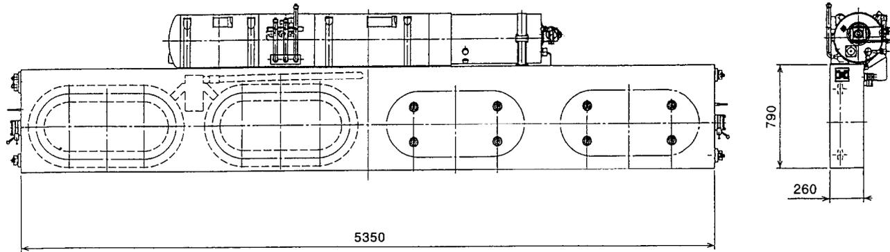
Figure 7 Illustration of the prototype superconducting magnet
