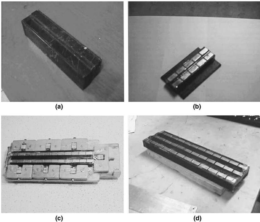
Fig. 2. Levitation rails: (a) Ferrite (rail 1), (b) Nd–Fe–B (rail 4), (c) Nd–Fe–B (rail 2) and (d) Nd–Fe–B, 3 lines (rail 3).
