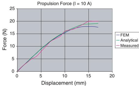
Fig. 4. Propulsion force for  $I_a = 10.0$  A.
