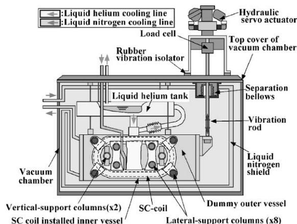
Fig. 1. Schematic of the vertical SC coil vibration test system.
