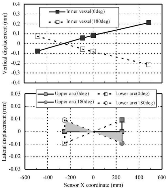
Fig. 2. An example of SC coil vibration mode under a vertical vibration.
