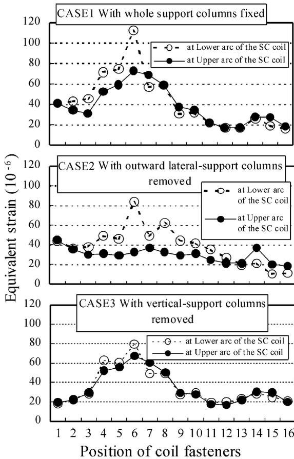
Fig. 5. Strain distributions of SC coil (FEM analysis results).
