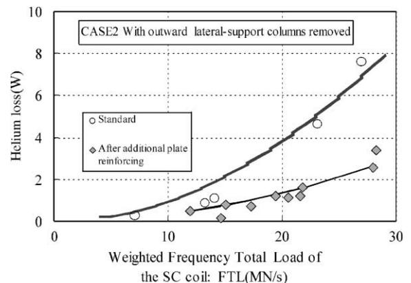
Fig. 7. A comparison of vertical SC coil vibration test results between standard and additional plate reinforcing inner vessels.
