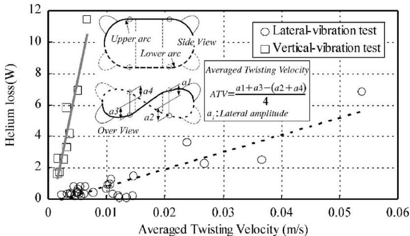
Fig. 3. Comparison of helium loss sensitivity to the SC coil twisting between lateral and vertical vibration test results.
