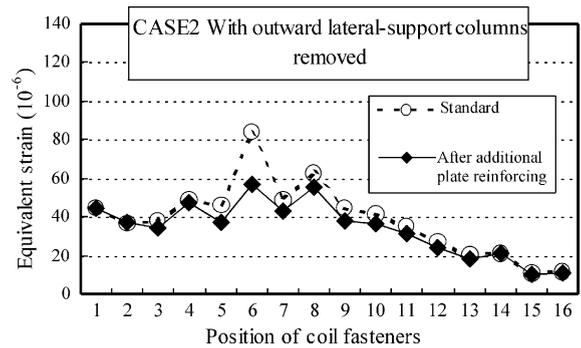
Fig. 6. A comparison of SC coil strain distributions between standard and additional plate reinforcing inner vessels.
