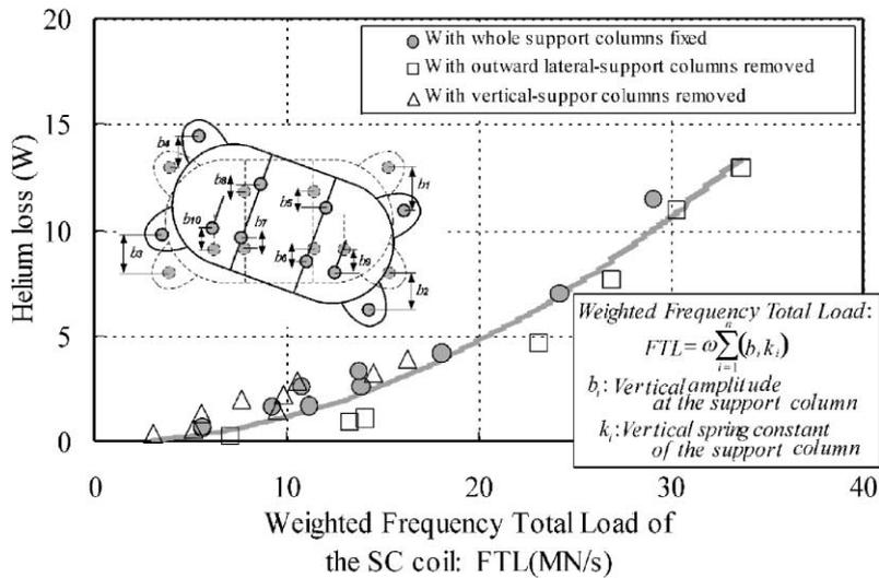
Fig. 4. Helium loss versus weighted FTL.
