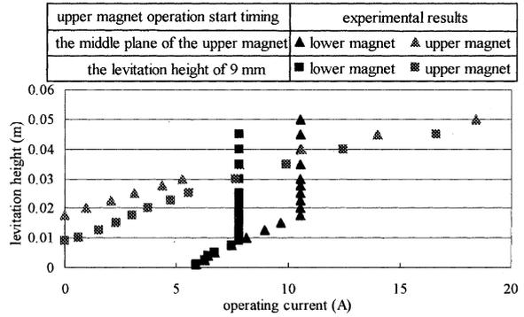
Fig. 5. Levitation height vs. operating current.
