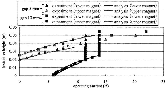
Fig. 3. Levitation height vs. operating current.
