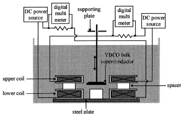
Fig. 1. Experimental setup for measurements of levitation height.
