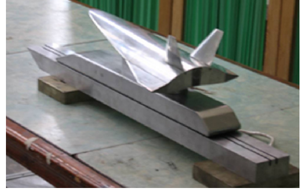
Fig. 2. Scale model of the Maglifter and the space vehicle.
