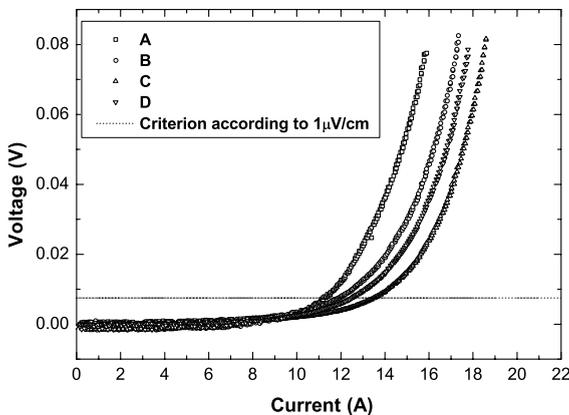
Fig. 8. Comparison of the voltage–current characteristics of the coil for different locations.
