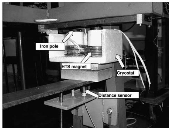
Fig. 2. Configuration of the magnetic circuit.
