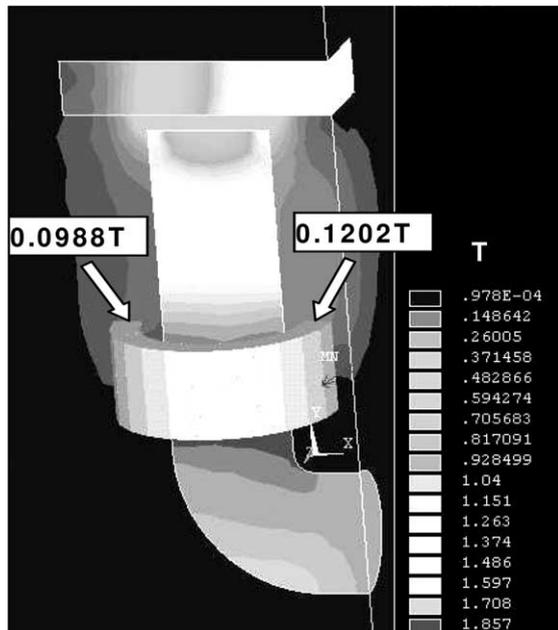
Fig. 6. Flux distribution in a coil with U-shape iron core. As a result of symmetry, only one quarter of the area is modelled. Here the value marked in the figure corresponds to value in the direction parallel to the  $X$ -axis. A symmetrical point is also selected for comparison.
