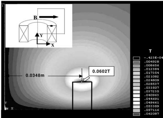
Fig. 5. Radial field distribution in the empty coil excited with current = 13.57 A. As a result of symmetry, only one quarter of the total area is modelled. The gray gradient in this figure represents the amplitude of the radial field.
