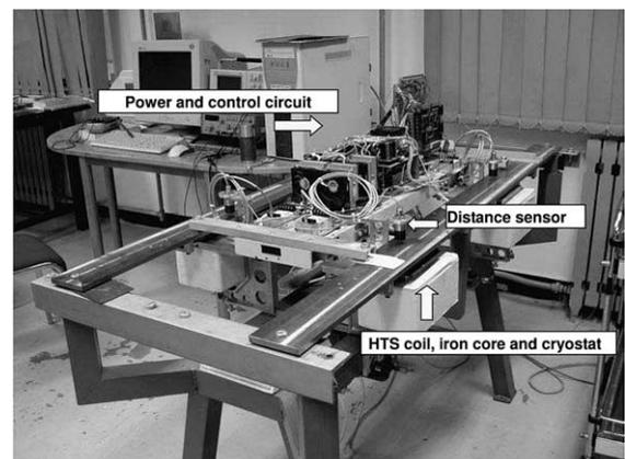
Fig. 1. Configuration of the EMS-based maglev vehicle.
