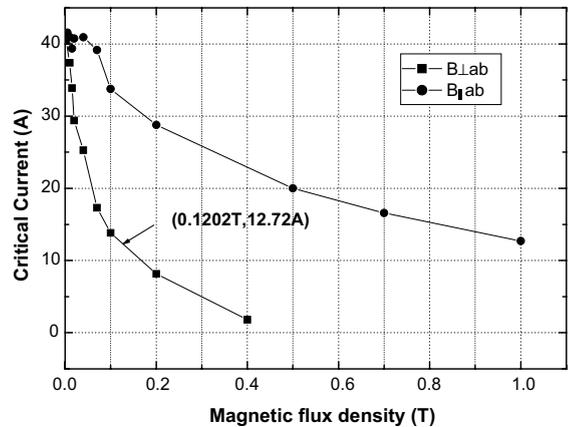
Fig. 3. Critical current as determined from short sample measurement as a function of applied field.
