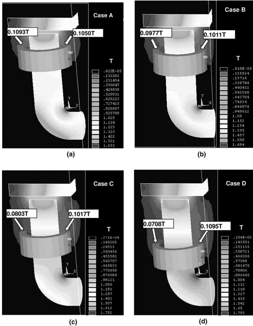
Fig. 10. Flux distribution of the magnetic circuit with coils located at different points. Note that the field marked in R1 and R2 corresponds to the field in the direction parallel to the X-axis.
