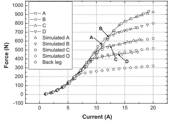
Fig. 9. Comparison of the force–current characteristics of the magnetic circuit for coils located at different points. The forces from A to D are 555, 641, 545 and 445 N, respectively. The simulation results for each case, as well as for the case of the coil placed at the back leg of iron core, are also shown.
