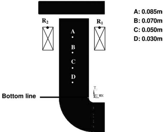
Fig. 7. Cross-section of the U-shape iron core showing the locations A, B, C and D, at different distances from the bottom line. Location D is used in the practical implementation. R1 and R2 are two reference points for field comparison.
