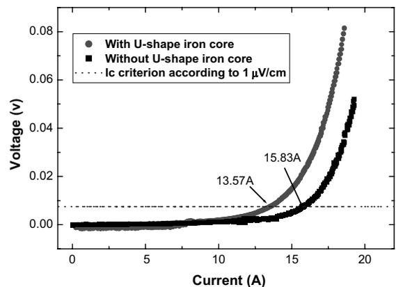
Fig. 4. Comparison of the voltage–current characteristics of the HTS coil with or without U-shape iron core.
