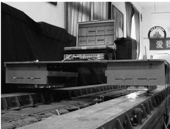
Fig. 2. The photo of the simplified HTS Maglev vehicle model in levitating.
