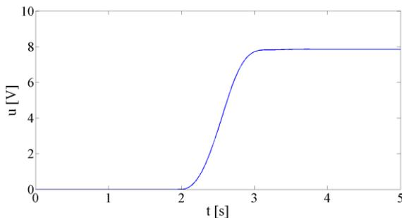
Figure 4. Control voltage signal applied to the electromagnet.
