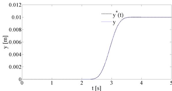
Figure 2. Closed loop position trajectory tracking response.
