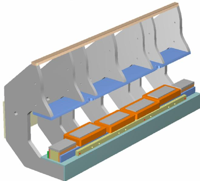
**Fig. 1. Magnet pod for  $M^3$  propulsion**
