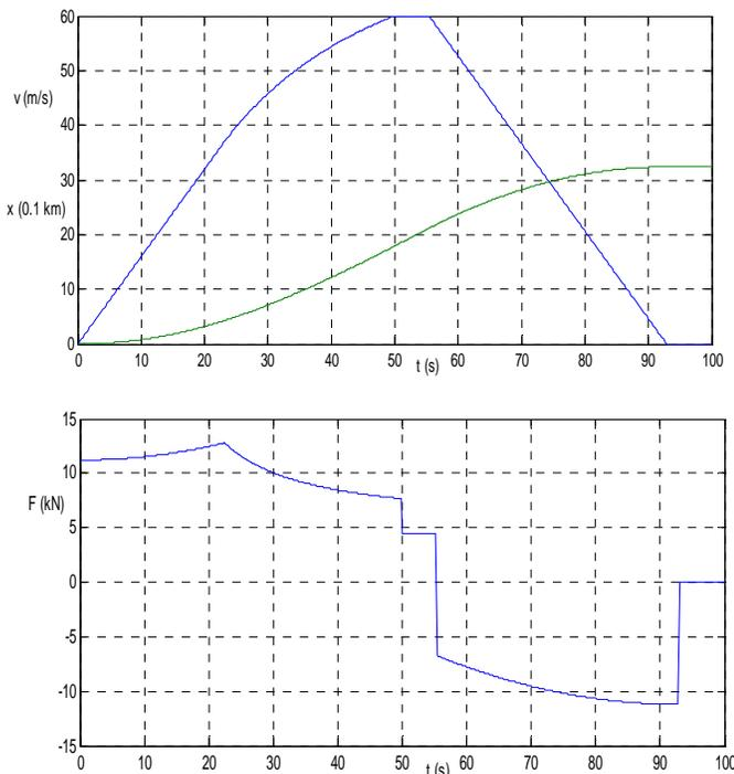
**Fig. 3. Distance, velocity and force vs. time.**
