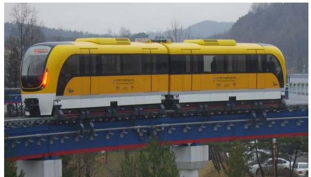
Figure 1. Maglev vehicle running over an elevated guideway
