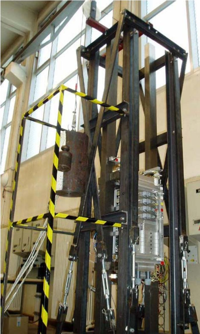
Figure 2. Electromagnetically guided elevator test bench.
