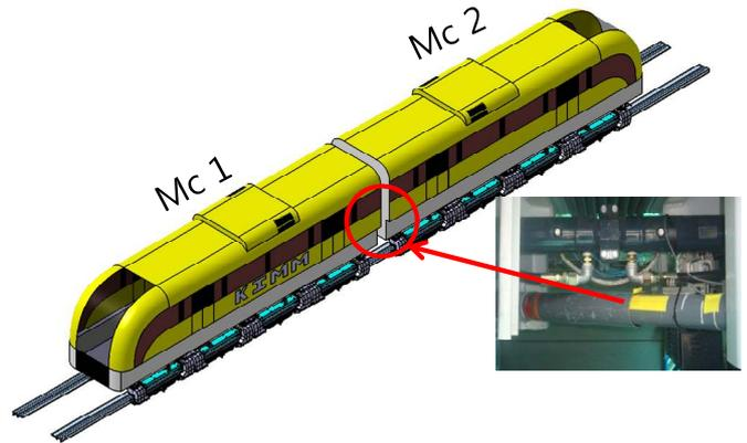
Figure 3. Dynamic full car model connected with damper
