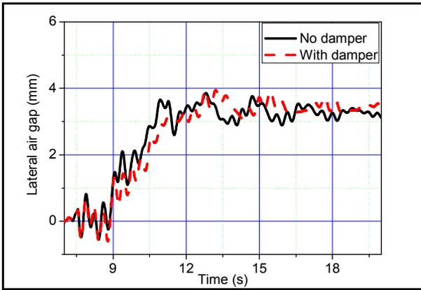
Figure 11. Lateral displacement of the bogie 4
