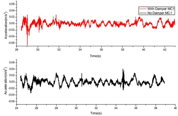
Figure 13. Lateral vibration running through test track, Mc 1
