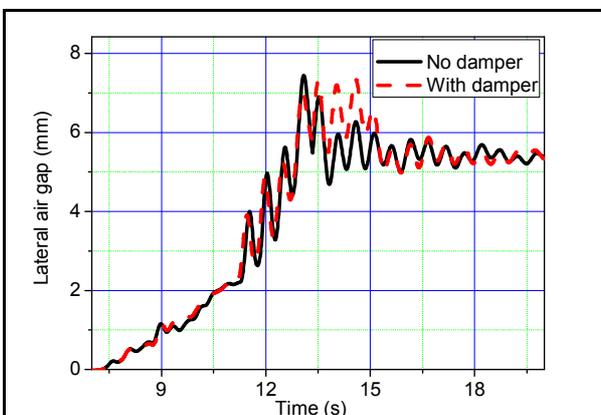
Figure 8. Lateral displacement of the bogie 4
