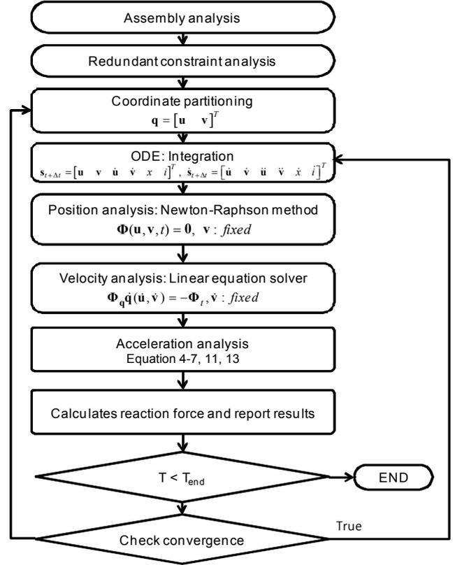
Figure 6. Numerical analysis flow
