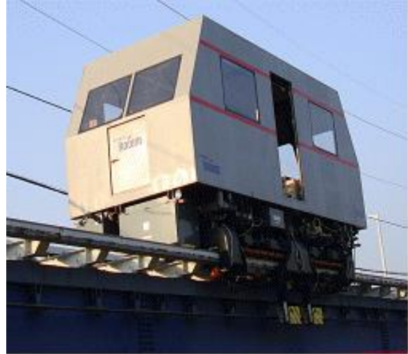
Figure 1. Experimental 1/2 Maglev vehicle.
