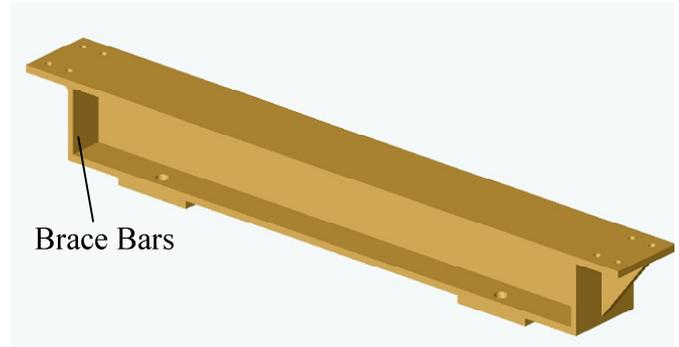
Figure 7. Reinforced sleeper by adding extra brace bars.
