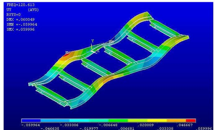
Figure 6. The second order modal shape of the track obtained by the FE method.
