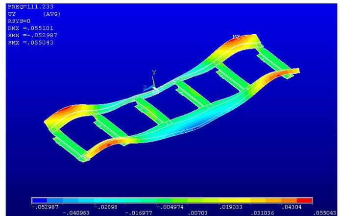
Figure 5. The first order modal shape of the track obtained by the FE method.
