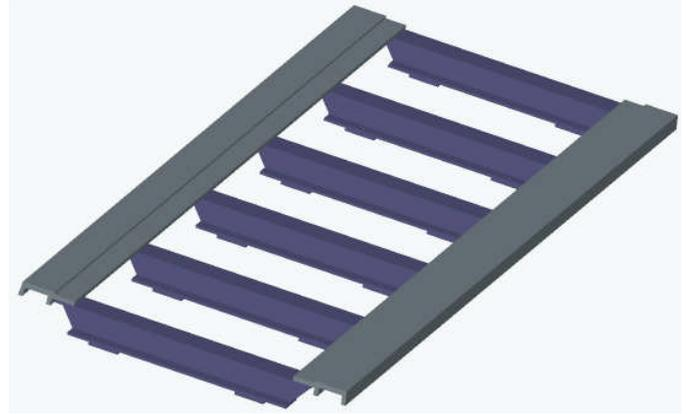
Figure 1. A segment of the low-speed maglev track.
