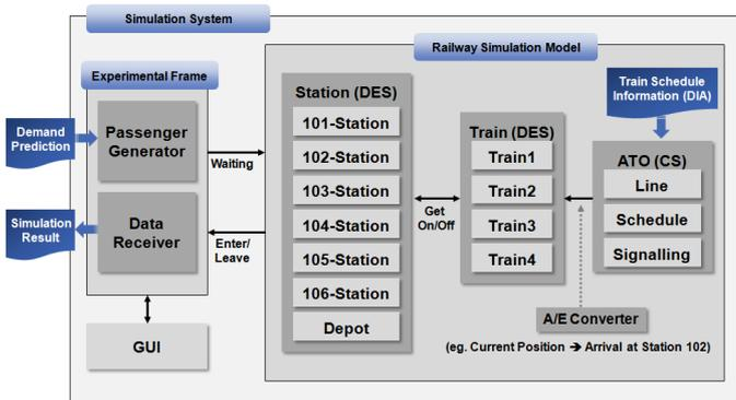
Figure 3. Detailed structure of the entire simulation system
