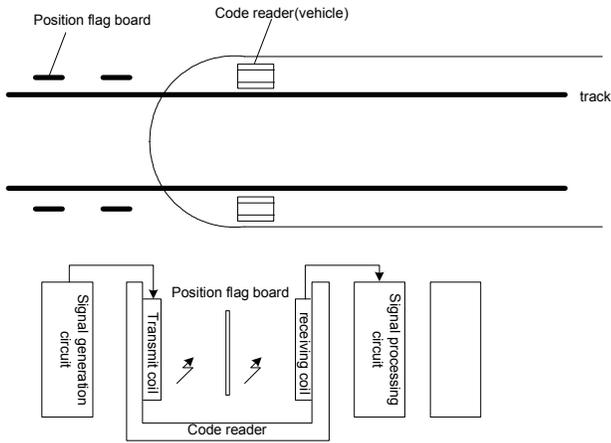
Figure 3. Topology of absolute position sensing system
