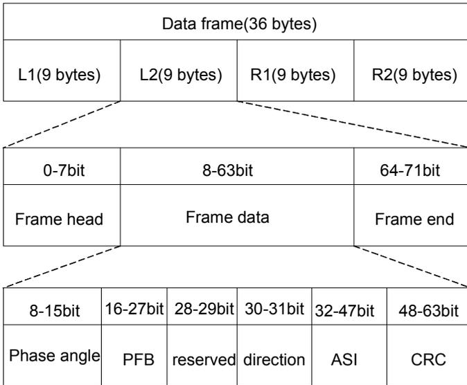
Figure 6. The coded data frame of position signal
