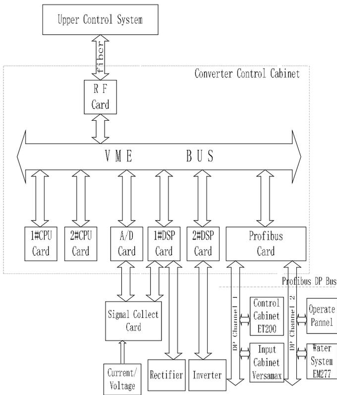
Fig1 Hardware Architecture of Digital Control System
