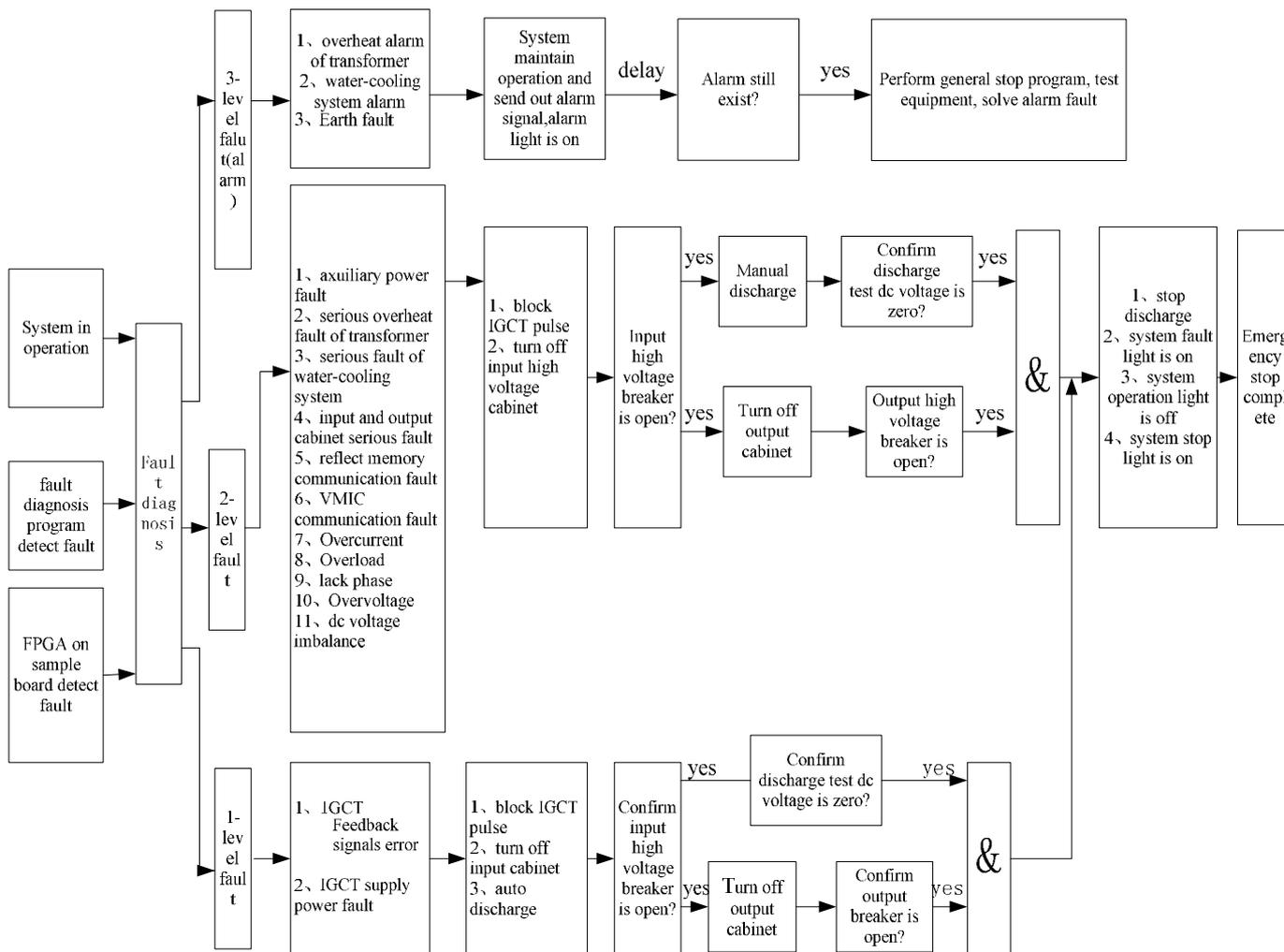
Fig.2 Faults Processing Flow
