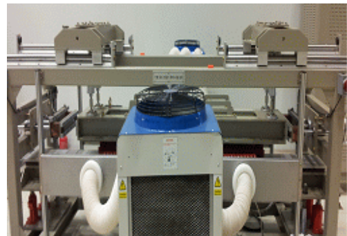
Figure.4 LIM test bed & Measuring device
