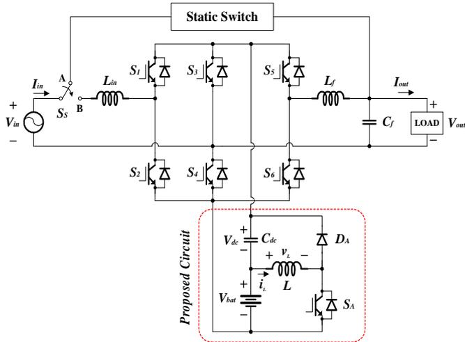
Figure 1. UPS with the proposed converter.
