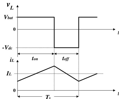
Figure 2. Key waveforms of the proposed converter.
