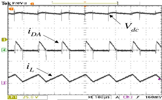
Figure 3. Key waveforms of the proposed converter.
