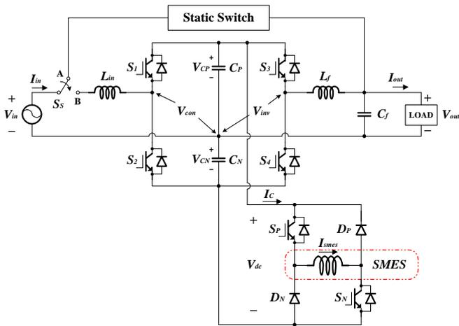
Figure 1. Proposed single-phase SMES-based UPS system.
