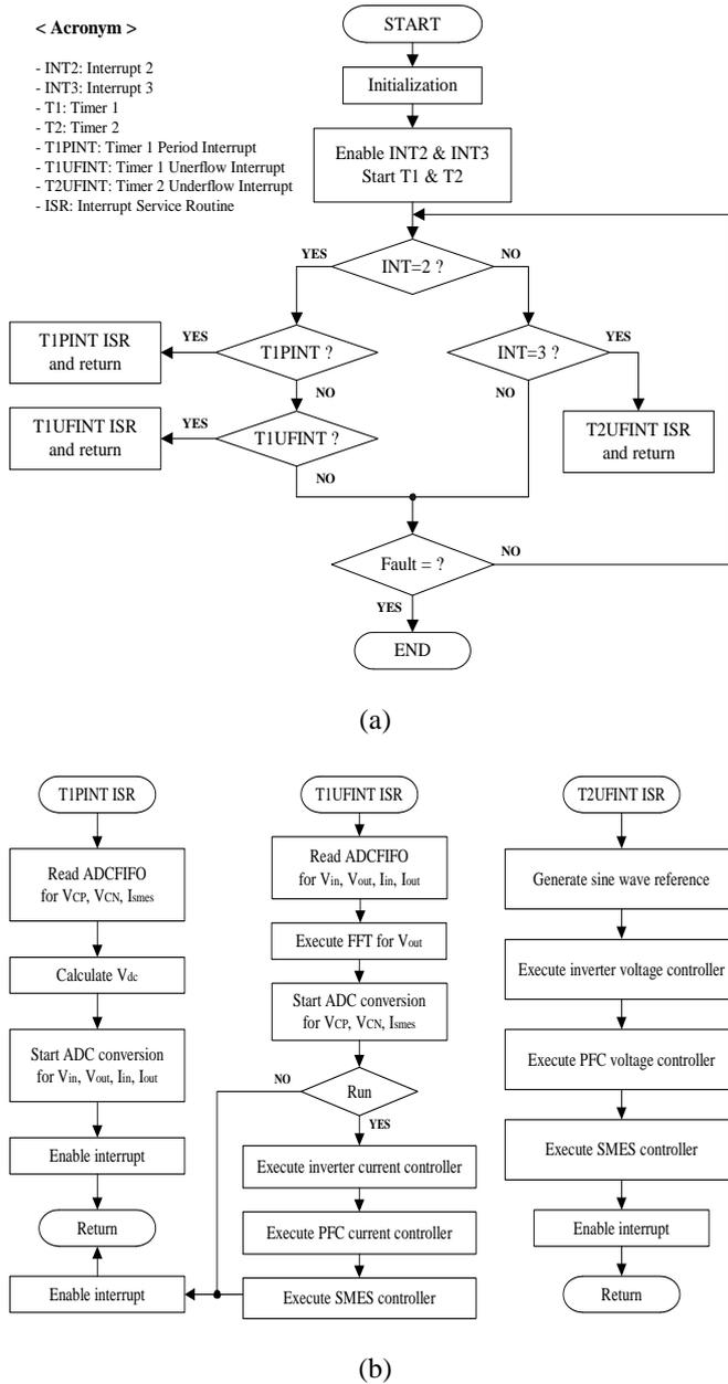
Figure 3. Software flowchart, (a) main program, (b) interrupt service routines.
