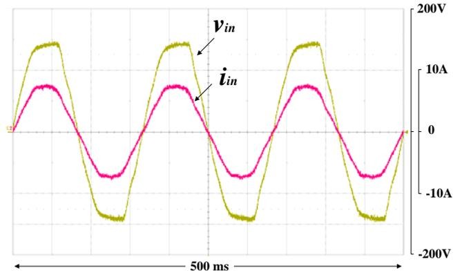
Figure 5. Input voltage and input inductor current at normal mode operation.
