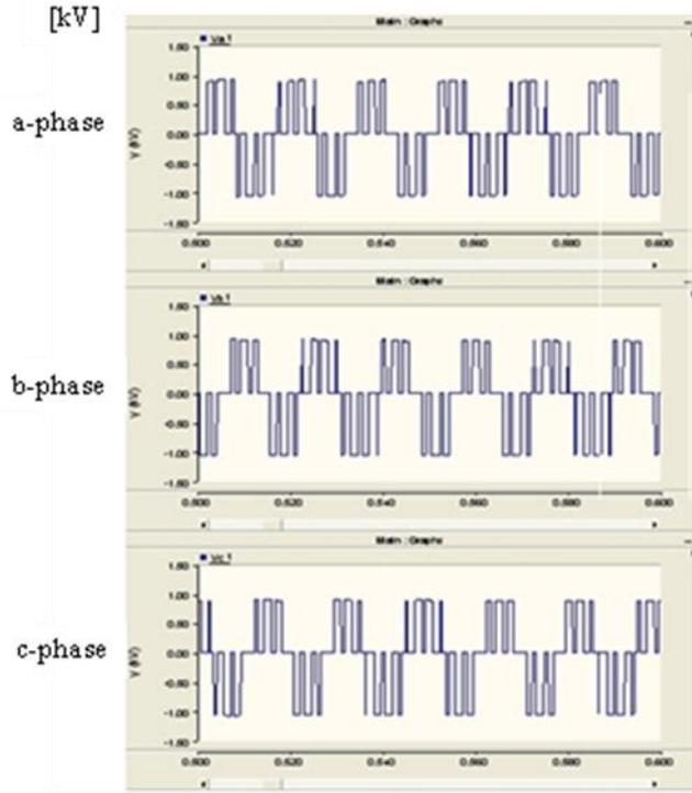
Figure 5. Waveform of phase voltages for inverter output
