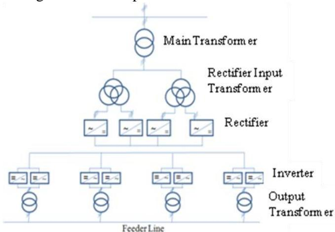
Figure 1. Power supply system.
