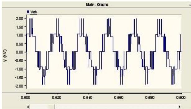
Figure 6. Waveform of Line-to-Line voltage for inverter output
