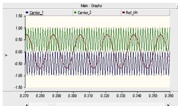
Figure 4. Waveform of standard wave and carrier waves
