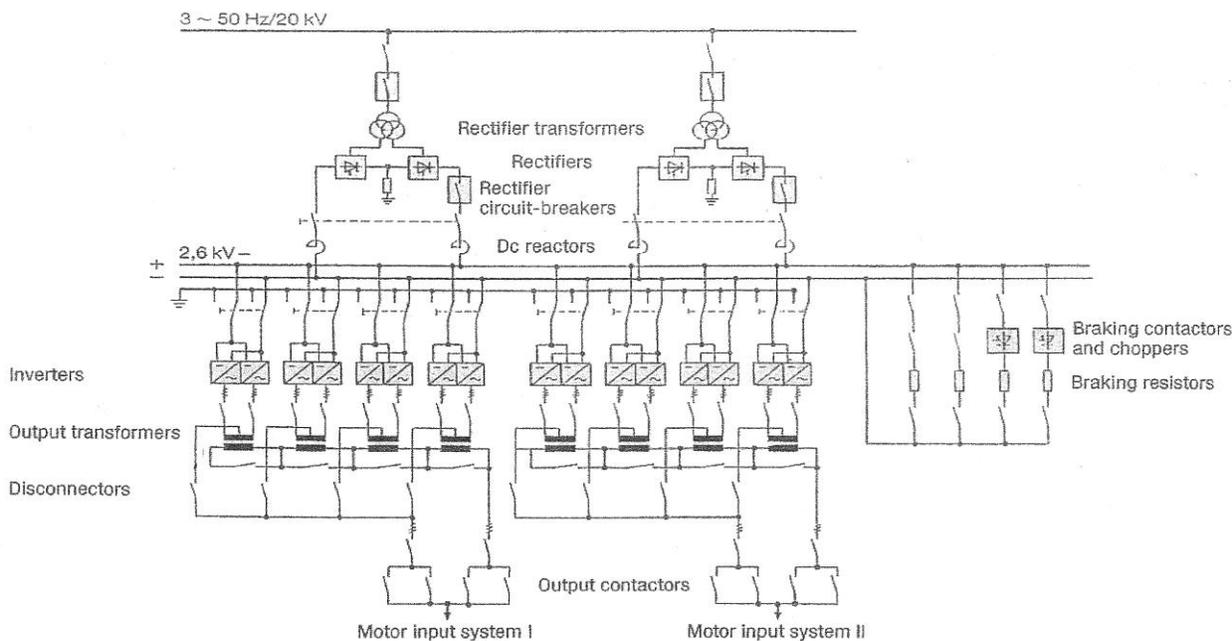
Figure 2. Power supply system for Transrapid 07[2].
