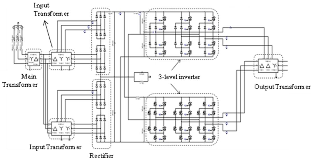
Figure 3. Modeling of power supply system using PSCAD/EMTDC
