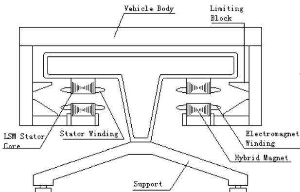
Figure 2. Cross section of the model vehicle
