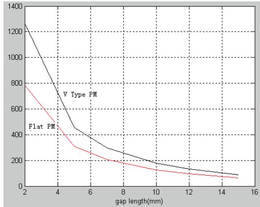
Figure 12. Lift force comparison
