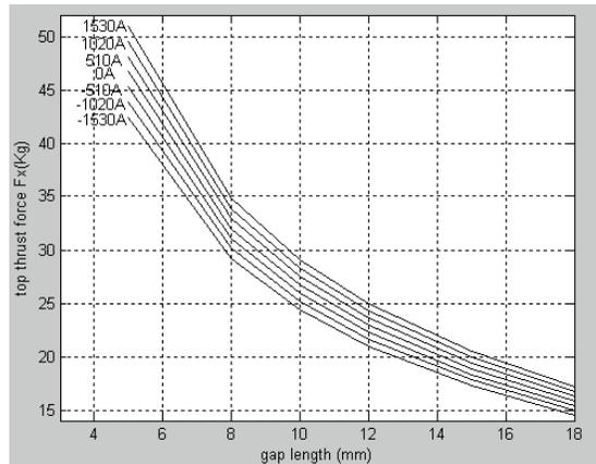
Figure 9. Maximum traction force (V type PM)
