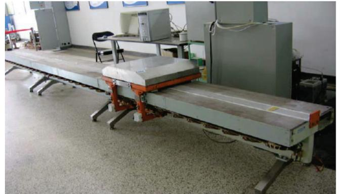
Figure 1. Hybrid levitation model vehicle in IEE, CAS.
