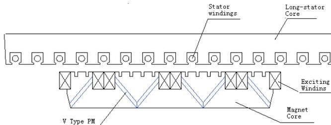
Figure 4. Structure of the LSM with V type PM (One unit of hybrid magnet)
