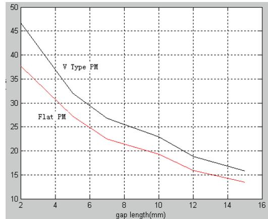
Figure 13. Maximum traction force comparison
