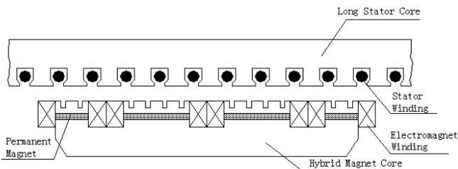
Figure 3. Structure of the LSM with flat PM (One unit of hybrid magnet)
