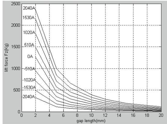
Figure 7. Lift force (V type PM)
