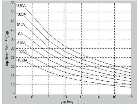
Figure 8. Maximum traction force (Flat PM)
