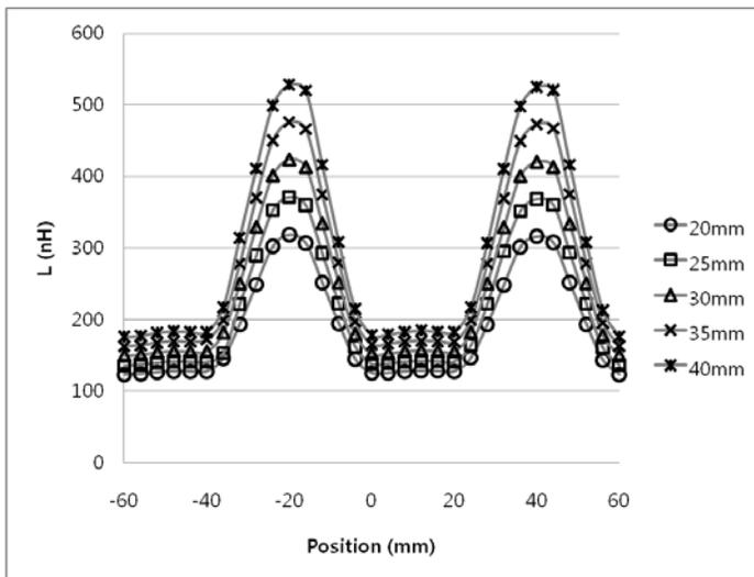
Figure 10. Leakage inductance of mover winding with different depth.
