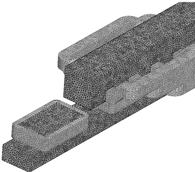
Figure 4. Mesh of the simulation model for finite element analysis.
