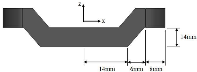
Figure 3. The end winding configuration of phase A winding. Phase B winding configuration is opposite in z direction.
