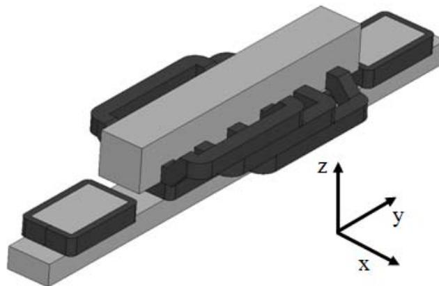
Figure 1. The geometry of the linear synchronous motor.
