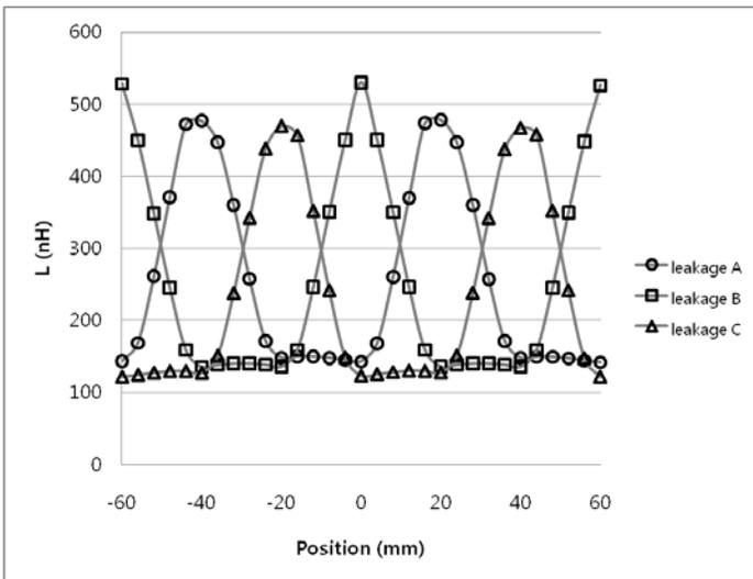
Figure 6. Leakage inductance of mover windings.
