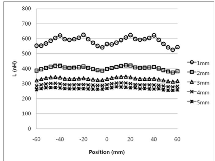
Figure 7. Self inductance of mover winding with different air gap.
