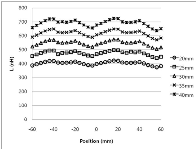
Figure 9. Self inductance of mover winding with different depth.
