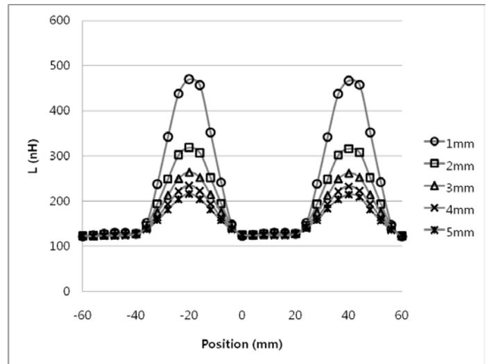
Figure 8. Leakage inductance of mover winding with different air gap.
