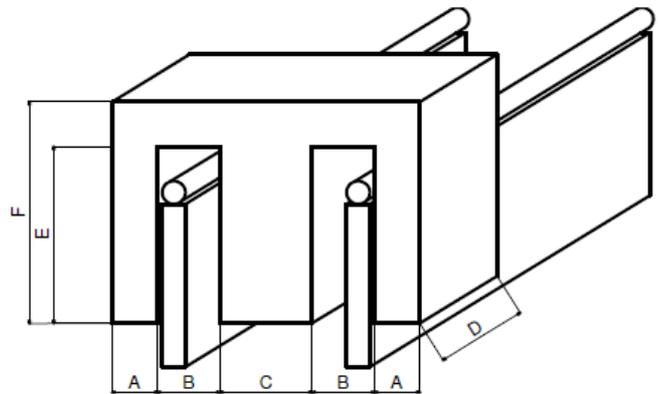
Figure 2. Contactless transformer segment 3D model.
