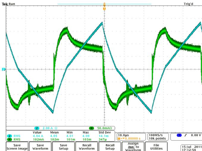
Figure 5. Input and output current of the RIPS's contactless transformer
