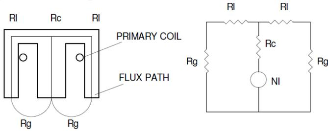
Figure 3. Flux path and magnetic circuit.
