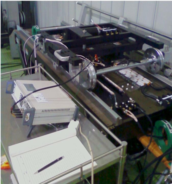
Figure 4. Measurement of the inductance of the secondary coil.
