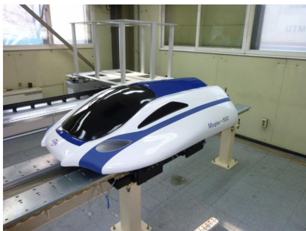
Fig. 22. Manufactured small scale magnetic levitation and propulsion system.
