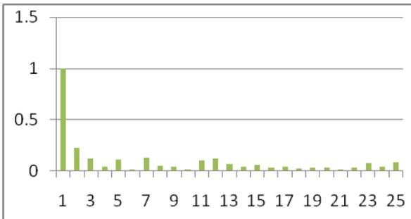
Figure 9 Harmonic content when 3.5MVA inductive load
