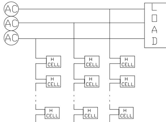
Figure 7 Cascaded H-bridge (CHB) Multilevel Converter
