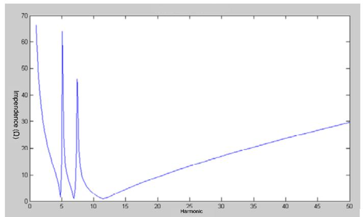
Figure 4 Filter impedance scan
