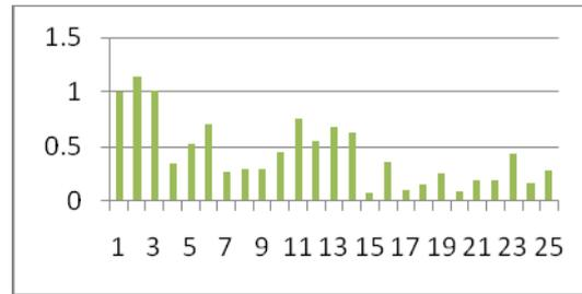
Figure 11 Harmonic content when no-load
