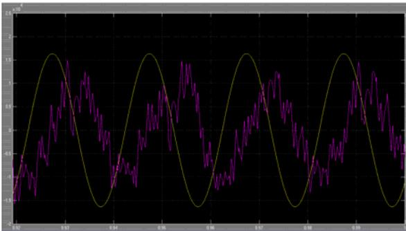
Figure 8 Output voltage and current when 3.5MVA inductive load
