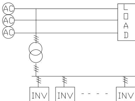
Figure 6 Multiple Three-phase Inverters in Parallel
