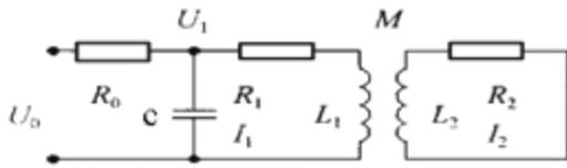
Figure 4. Equivalent detection circuits for the sensor
