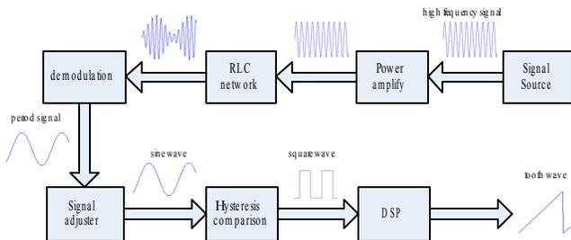
Figure 5. Signal processing circuit
