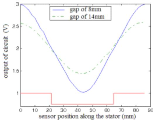
Figure 9. Output of detection circuit with different gap
