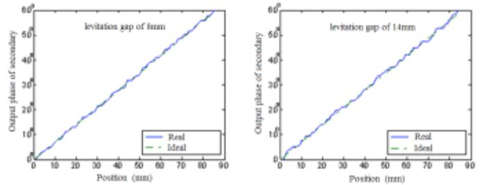
Figure 11. Experiment of position detection with different gaps
