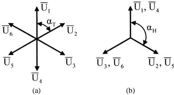
Figure 2. 6-phase system of the inverter output voltages:
