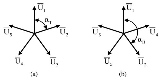
Figure 1. 5-phase system of the inverter output voltages:
