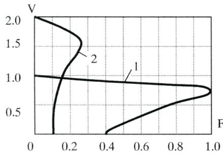
Figure 3. Mechanical characteristics of a multiphase linear inverter-fed induction motor on a per-unit basis: (1) natural characteristic, when the traditional control method is used ( $H = 1$ ), and (2) when OSM is used ( $H = 2$ ).
