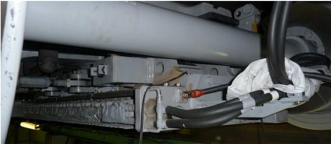
(b) Primary of a linear induction motor under study.
