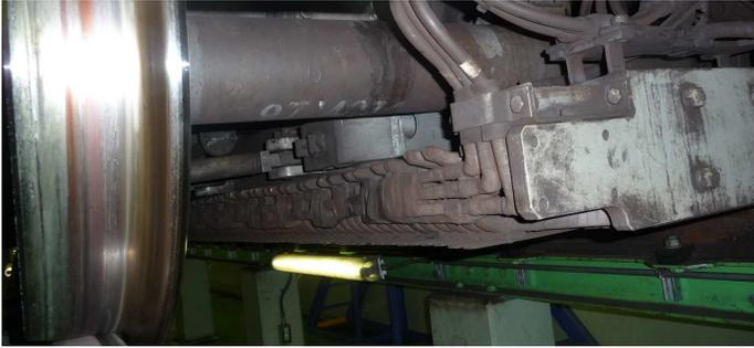
(a) Primary of a conventional linear induction motor.
