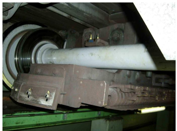
Figure 4. Primary of a linear induction motor for Oedo-Line.
