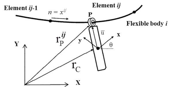
Figure 2. Sliding joint moving on a flexible body.
