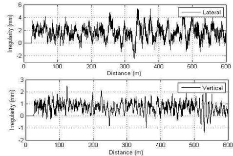
Figure 6. Lateral and vertical irregularities of the rail.
