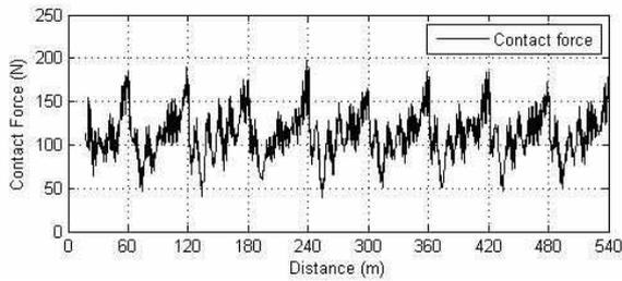
Figure 11. Contact force between contact wire and pantograph.
