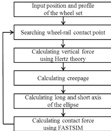
Figure 5. The process of the calculating contact force.
