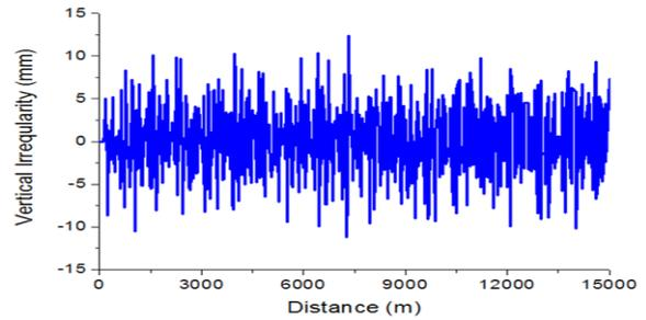
Figure 5. Vertical irregularity of the test track
