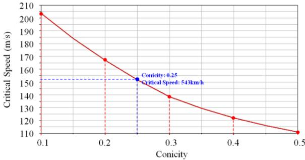
Figure 7. Stability analysis result (Conicity vs. critical speed)
