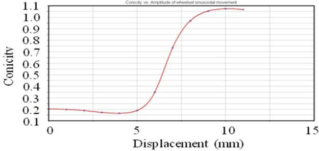
Figure 3. Conicity vs. wheelset sinusoidal movement
