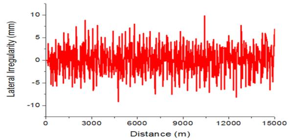
Figure 4. Lateral irregularity of the test track
