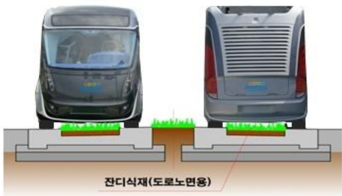
Fig. 5. Dedicated lanes covered with grass between left and right wheels
