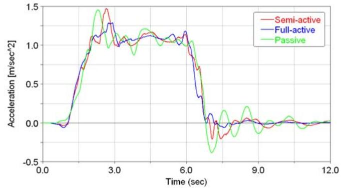
Figure 7. Lateral accelerations of rear end of car-body
