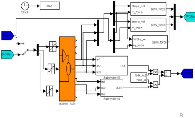
Figure 5. Simulation model of steering system with vehicle
