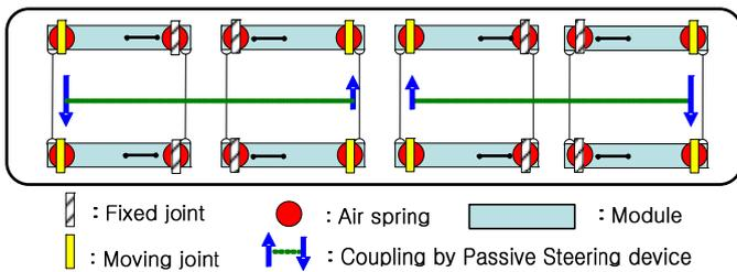
Figure 2. Schematics of passive steering system of target vehicle
