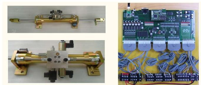
Figure 8. Proto-type of semi-active actuator and controller
