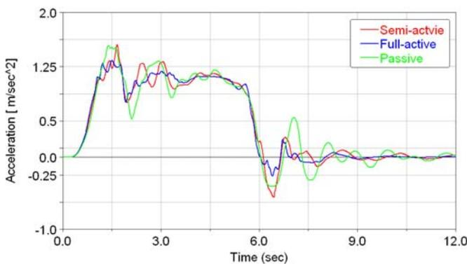
Figure 6. Lateral accelerations of front end of car-body
