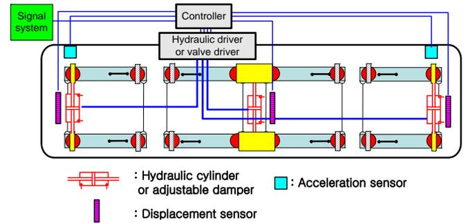
Figure 3. Schematics of active steering system
