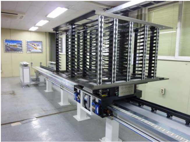
Figure 1. Maglev conveyor system.
