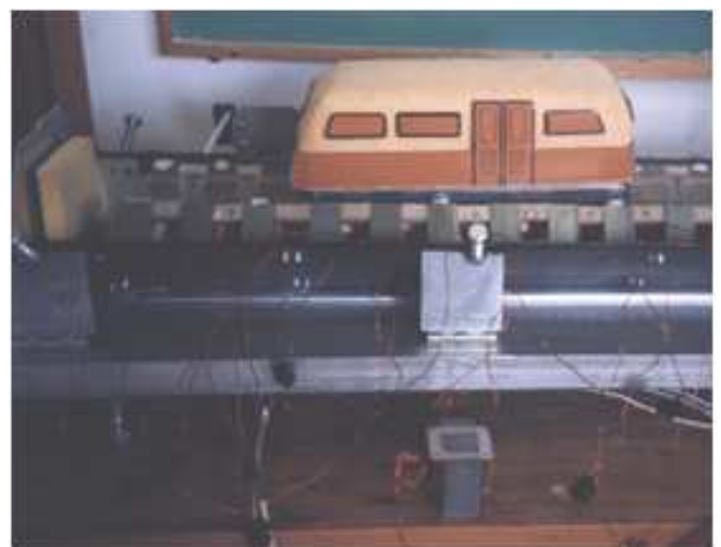
Figure 16. Prototype of an EDL people mover suspended, propelled and stabilized using a V-shaped LIM.
