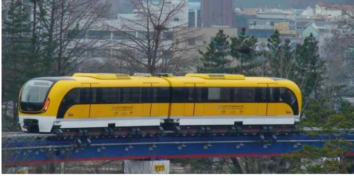
Figure 3. Prototype Maglev Trainset on Test Track
