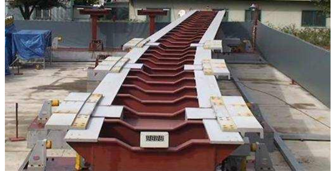
Figure 4. Three Way Articulated Turnout
